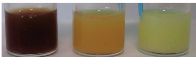
Figure 6. Structure and colloidal suspensions of N-doped \text{TiO}_2 NPs. (a) X-ray diffraction diagrams (Cu K\alpha ) as a function of the annealing temperature for \text{TiO}_2 NPs. Peaks correspond to the anatase type structure. (b) Photographs of aqueous suspensions containing N-doped \text{TiO}_2 NPs annealed 2 h at 700 °C under \text{NH}_3 (left), then heated 2 h in air at 300 °C (left), at 400 °C (middle), or 500 °C (right).
